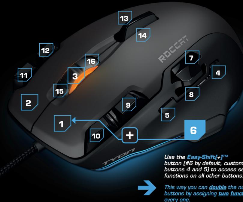
Use the **Easy-Shift[+]™** button (#6 by default, customizable to buttons 4 and 5) to access second-level functions on all other buttons.
